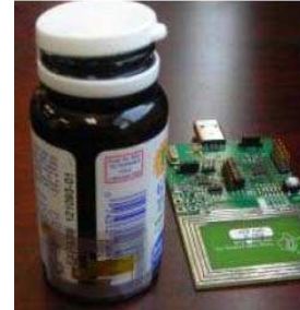
Figure 5: RFID reader and RFID tags on a bottle
